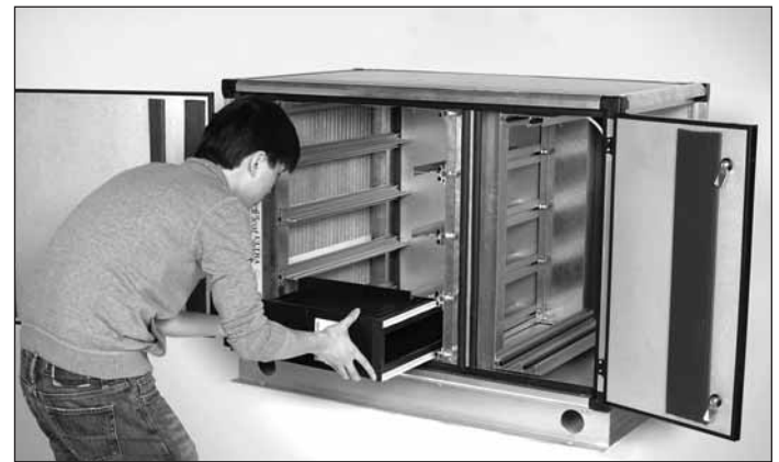
Step 3: Rotate the cassette slightly so that the vertical locator bars are inserted into the slots in the half-cassette while maintaining the compression between the hollow core and butterfly gaskets. See Detail 1 – Step 3 and Detail 2 – Step 3.
