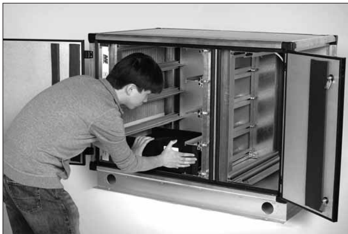
Step 4: Maintaining a steady and even force on the side of the cassette push it into the housing to engage the notches on the outer side of the half-cassette and continue to insert the half-cassette until it is fully installed.
