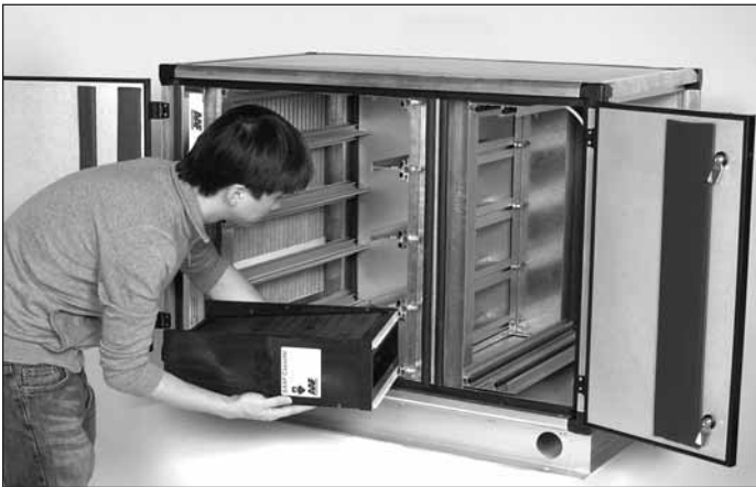
Step 2: Engage the upper and lower black hollow core gaskets in the tracks with the yellow butterfly gaskets on the half-cassette, see Detail – Step 2. Also, begin to align the upper and lower notches in the half-cassette with the vertical cassette locator bars which form part of the track.
